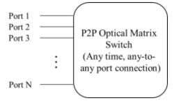
The 360 series Optical Matrix Switch comprises N equivalent optical fiber ports (total port count customizable based on requirements), allowing any two ports to be interconnected at any given time.
